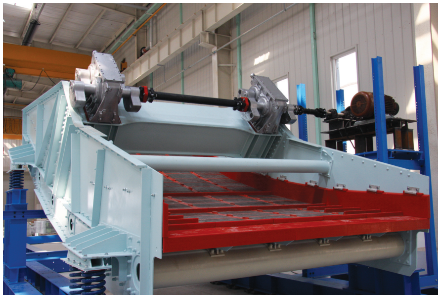
ABS3673 Single deck banana screen on a test frame (top), the distinctive red polyurethane plug, an Aury screen trademark (left)
